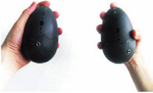
Figure 1. Two Mobile Feelings interface devices that enable users to wirelessly transmit and receive each others' heartbeat and breath.
